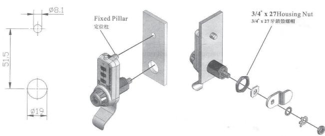
VI、When the finger pull is not installed, please add one flat washer to assist the lock to fix 不裝把手時,搭配一顆平華司
