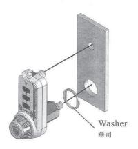
VII · Please note, before installing the cam, please turn the wheels to the correct combination code, and then tighten the cam by hex nut. Please comply with these steps when installing to ensure the internal components functions normally."
